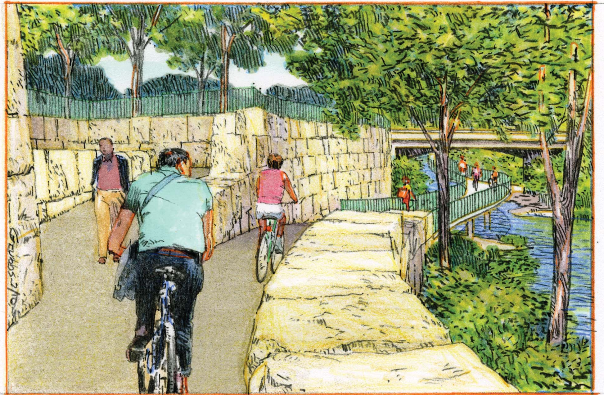
The existing stone retaining walls and switchback ramp south of the Cesar Chavez Bridge will be restored as part of the trail system and linked with an elevated boardwalk structure to the north.
