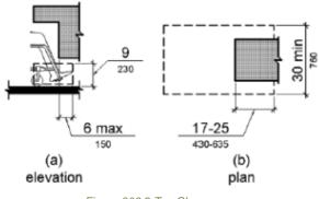
Figure 306.2 Toe Clearance
