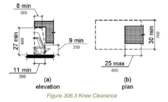
306.3.2 Maximum Depth. Knee clearance shall extend 25 inches (635 mm) maximum under an element at 9 inches (230 mm) above the finish floor or ground.
