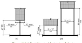
Figure 307.3 Post-Mounted Protruding Objects
