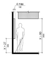
Figure 307.2 Limits of Protruding Objects
