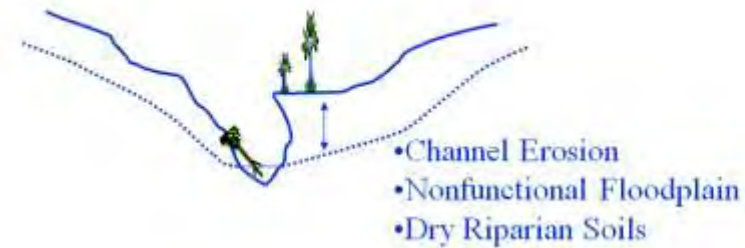
Channel with Incision Due to Increased Runoff
